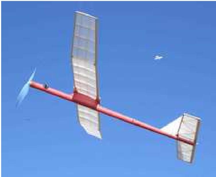
This is a relatively modern design from Europe. Note the tapered rolled tube fuselage.
