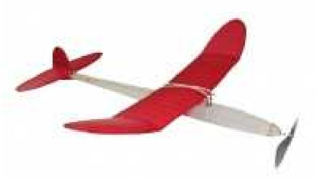
This P-30 has the classic appearance of an Old Time Rubber stick model. It has a parasol mounted wing with elliptical shaped tips.
