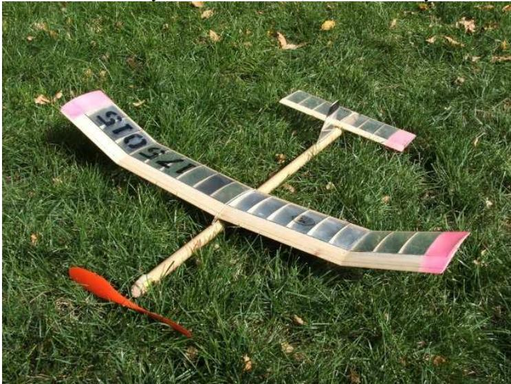
This perennial winner at the AMA Nats has a D-box under-cambered wing with carbon fiber reinforcements.
