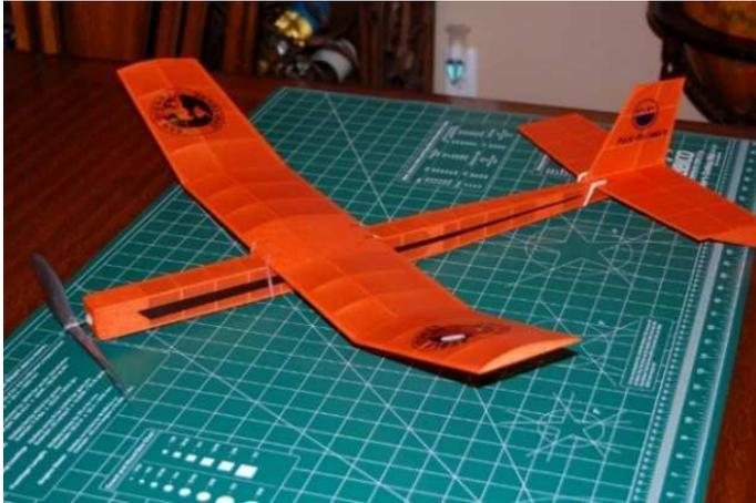
This basic 28-inch wingspan model was formerly sold by Peck-Polymers for many years under the name One Nite 28. It doesn't accommodate a blast tube with a conventional outside diameter.
