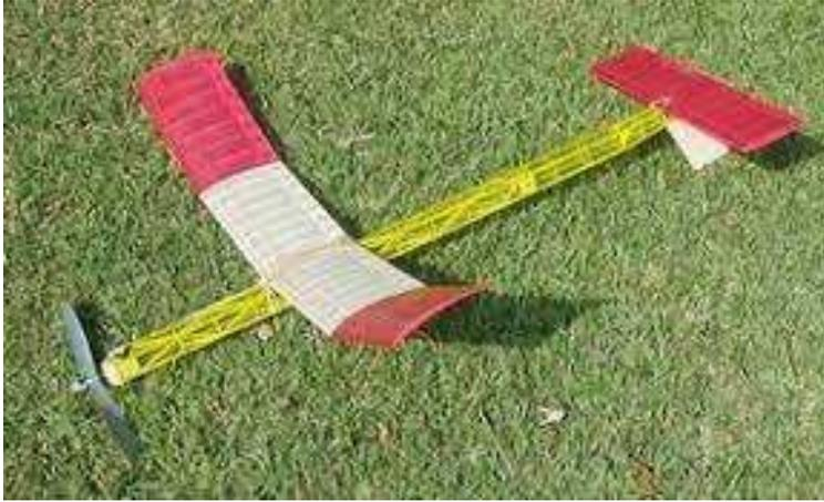
This P-30 design from South America has achieved many contest victories. The wing has a very thin undercambered airfoil. Note the unusual fin location beneath the stab.
