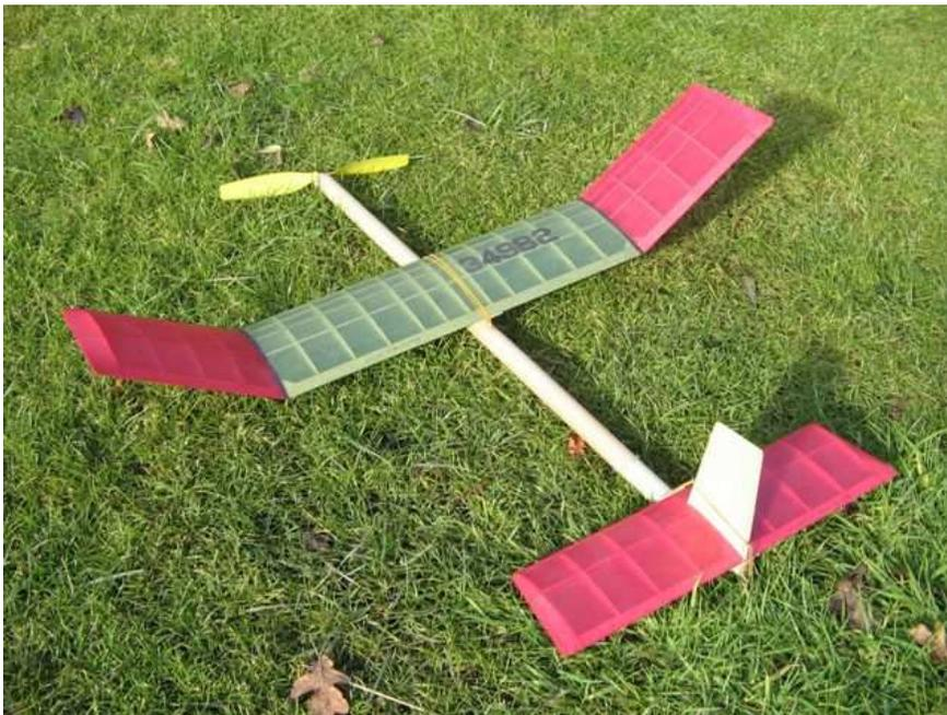
A stick and tissue P-30 model with a rolled tubular fuselage supplied with the kit. This design appears similar to the Pee-Wee and Polecat in overall configuration.
