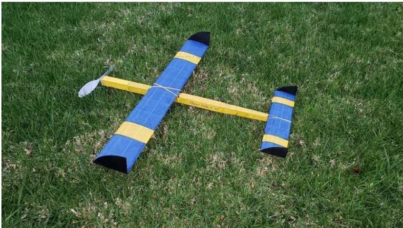
The author's own P-30 design was first introduced in 2021. It is the easiest and quickest P-30 to construct due to its unique configuration that includes a flat wing with tip plates. I won the 2021 John Oldenkamp Memorial P-30 contest (in the third round of the fly off) flying my red and yellow tissue covered Three Nite P-30. The one shown above was lost OOS on a trim flight and was not recovered.
