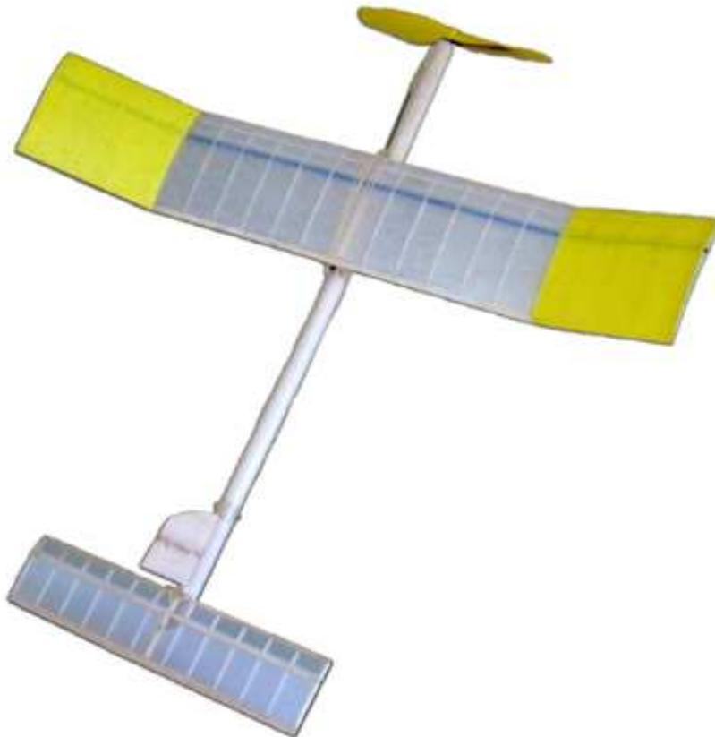
This is a proven consistent winner designed and flown by an expert for three decades. Note the carbon fiber composite main spar in the wing.
